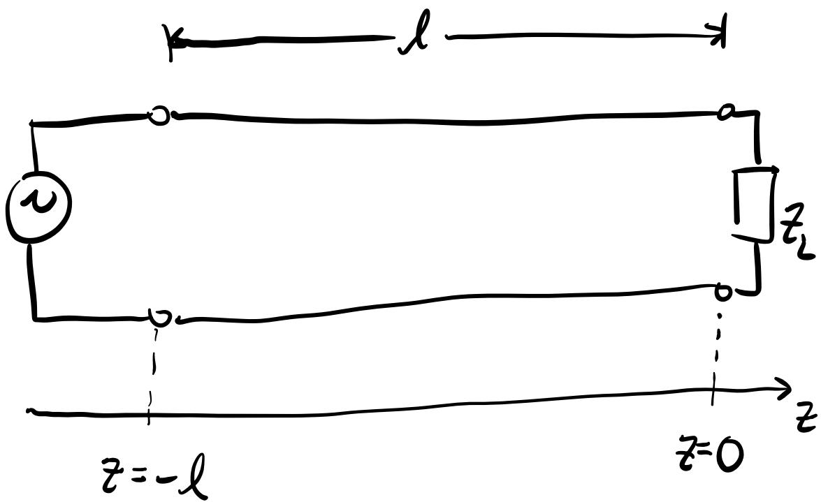
With the chose coord. system, the voltage & current amp. at the pos. of  $Z_L$  ( $z=0$ ) are given by :
